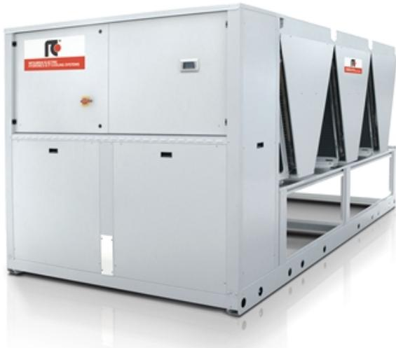
**Outdoor unit for the production of chilled water with hermetic rotary Scroll compressors, ozone-friendly refrigerant R410A, axial-flow fans, braze-welded plate-type heat exchanger, micro-channel full-aluminum air coils and thermostatic expansion valve. The range is composed by units equipped with four compressors in tandem configuration on two independent refrigeration circuits.**
