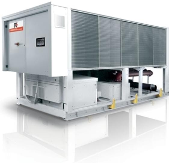
Outdoor unit for the production of chilled water, equipped with oil-free centrifugal compressors, R134a refrigerant, axial EC fans, condensing coil with copper tubes and aluminum fins, shell and tube flooded evaporator and electronic expansion valve. Base, supporting structure and panels are of galvanized epoxy powder coated steel; the unit is supplied with refrigerant.
