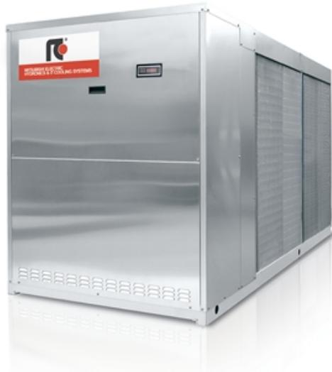
Outdoor unit for the production of chilled water with hermetic rotary Scroll compressors, axialflow fans, shell and tubes exchanger and thermostatic expansion valve. External panels in Peraluman and structure in aluminium sections. The range is equipped with two compressors on two independent refrigerant circuits.
