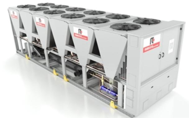
Outdoor unit for the production of chilled water with semi-hermetic variable-speed screw compressors optimized for R134a, axial-flow fans, micro-channel full-aluminum condensing coils, single-pass shell and tubes evaporator designed by Mitsubishi Electric Hydronics & IT Cooling Systems S.p.A. and electronic expansion valve.
