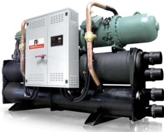
**High efficiency unit for indoor installation for chilled water production. Semihermetic screw compressors optimized to operate with low compression ratio and R134a; shell and tubes condenser, flooded evaporator and electronic expansion valve. High efficiency unit thanks to the innovative optimized compressors and the high performing heat exchangers.**
