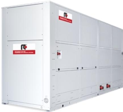
Unit for indoor installation to produce chilled water with hermetic rotary Scroll compressors, centrifugal plug fans with EC motor, braze-welded plate-type exchanger and thermal expansion valve.
