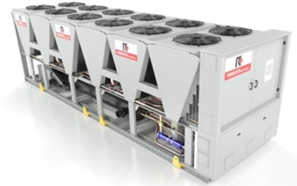
Outdoor unit for the production of chilled water with semi-hermetic variable-speed screw compressors optimized for R513A, axial-flow fans, micro-channel full-aluminum condensing coils, single-pass shell and tubes evaporator designed by Mitsubishi Electric Hydronics & IT Cooling Systems S.p.A. and electronic expansion valve.
