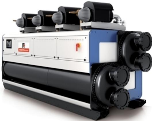
**Indoor unit for the production of chilled water featuring centrifugal compressors oil-free, with R134a, electronic regulation valve, shell and tube condenser and shell and tube flooded evaporator.**
