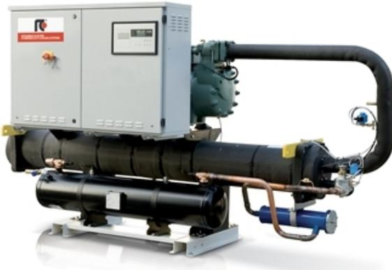
**Indoor unit for the production of chilled water combined with a remote condenser, with semi-hermetic screw compressors optimized for R134a, shell and tube evaporator designed by Mitsubishi Electric Hydronics & IT Cooling Systems S.p.A. and thermostatic expansion valve.**
