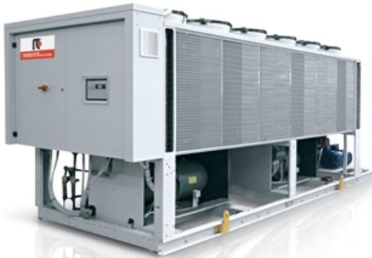
Outdoor unit for the production of chilled water, equipped with semi-hermetic screw compressors, R513A refrigerant, axial-fans, condensing coil with copper tubes and aluminum fins, shell and tube evaporator single pass and electronic expansion valve. Base, supporting structure and panels are of galvanized epoxy powder coated steel. The unit is supplied with anti-freeze oil and refrigerant and has been factory tested.
