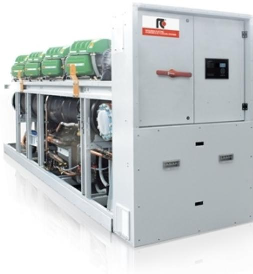
**Indoor unit for the production of chilled water featuring centrifugal compressors oil-free, with refrigerant HFO (1234-ze), electronic regulation valve, shell and tube condenser and shell and tube flooded evaporator. Base and supporting structure and panels are of galvanized epoxy powder coated steel with increased thickness.**
