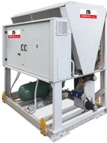
Outdoor unit for the production of chilled water with semi-hermetic screw compressor optimized for R513A, axial-flow fans, micro-channel full-aluminum condensing coils, single-pass shell and tubes evaporator designed by Mitsubishi Electric Hydronics & IT Cooling Systems S.p.A. (brazed plate evaporator for sizes 0751 and 0851) and electronic expansion valve. Base and supporting structure and panels are of galvanized epoxy powder coated steel with increased thickness. Eurovent certification.
