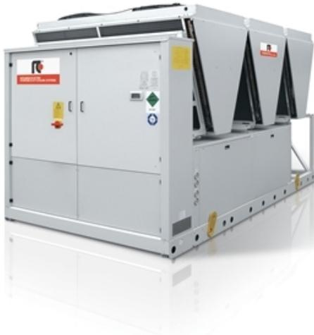
Outdoor unit for the production of chilled water with hermetic rotary Scroll compressors, ozone-friendly refrigerant R410A, axial-flow fans, shell and tubes exchanger and electronic expansion valve. The range is composed by units equipped with four, six and eight compressors in multi-circuit configuration.
