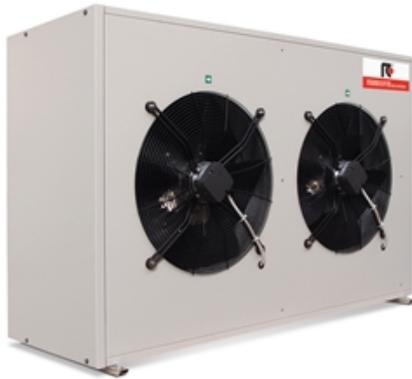
Remote condensers with axial-type fan(s) for outdoor installation. Installation may be vertical with a horizontal air outflow or, using special brackets, horizontal with an upward air outflow. The very low noise, adjustable-speed fans are excellent for use in both technological and civil applications. The units operate with a single-phase 230V/1ph/50Hz and 400V/3ph/50Hz and are fitted with integrated fans speed regulator per standard.
