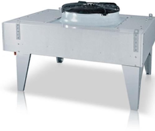
Remote condensers with axial-type fan(s) for outdoor installation. Installation may be vertical with a horizontal air outflow or, using special brackets, horizontal with an upward air outflow. The EC motor fans with very low noise and adjustable-speed fans are excellent for use in both technological and civil applications. Remote condensers are not provided with integrated fans speed regulator per standard. However, it can be supplied as OPTIONAL and installed directly inside the indoor unit.
