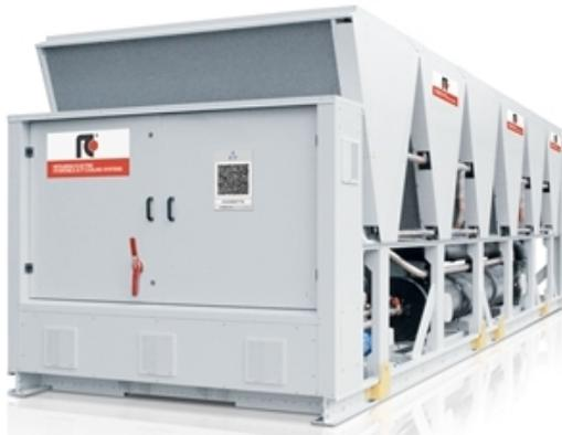
**Outdoor unit for the production of chilled water with semi-hermetic screw compressors optimized for HFO refrigerant R1234ze, axial-flow fans, micro-channel full-aluminum condensing coils, single-pass shell and tubes evaporator designed by Mitsubishi Electric Hydronics & IT Cooling Systems S.p.A. and electronic expansion valve.**
