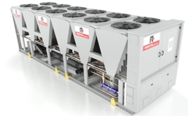
Outdoor unit for the production of chilled water with semi-hermetic variable-speed screw compressors optimized for HFO R1234ze refrigerant, axial-flow fans, micro-channel full-aluminum condensing coils, single-pass shell and tubes evaporator designed by Mitsubishi Electric Hydronics & IT Cooling Systems S.p.A. and electronic expansion valve.
