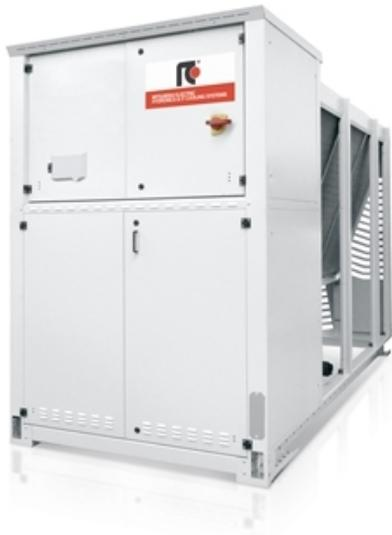
Outdoor unit for the production of chilled water with fixed speed and variable speed (Inverter Driven) Scroll compressors, optimized for R410A in a single-circuit configuration, axial-flow fans, micro-channel full-aluminum air coils and electronic expansion valve as standard equipment.
