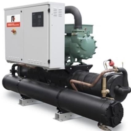
Indoor unit for the production of chilled water featuring semihermetic screw compressors optimized to operate with low compression ratio, refrigerant HFO R1234ze, shell and tubes evaporator designed by Mitsubishi Electric Hydronics & IT Cooling Systems S.p.A. and shell and tube condenser and electronic expansion valve.
