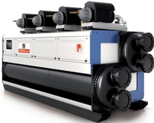
**Indoor unit for the production of chilled water featuring centrifugal compressors oil-free, with R513A, electronic regulation valve, shell and tube condenser and shell and tube flooded evaporator.**
